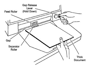
After the thick document(s) have been scanned, release the gap release lever. It will return to its original position. The feed and separator rollers will return to their previously adjusted positions.
